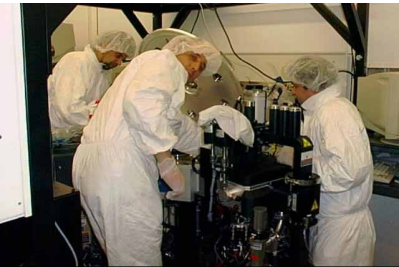
Equipment integration Integration of your process equipment under clean room conditions, connection of all media and start up
